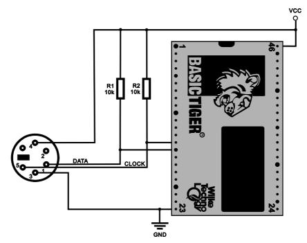
Since an MF-II keyboard does not send ASCII-codes, but requires further steps of code conversion, quite complex measures are necessary to get the desired keyboard function. As a basis, and in addition to the sample program, several include-files are provided as well, that can be adjusted to individual needs. MF2\_TR.INC is the only include file to be integrated into the application. MF2\_TR.INC itself integrates all further include files.
