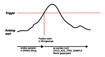
Measuring with trigger is restricted to strings and not possible with FIFO !!!
