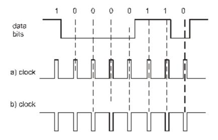
On the Tiger 2<sup>®</sup> modules, the cycle time is 1.4 microseconds as a standard. With SET\_SYSVARN, a system variable can be set that slows down the clock, up to a cycle time of 5.8 microseconds.
