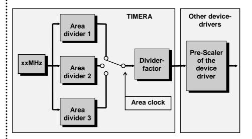
Further information about setting the device-driver TIMERA can be found in the description of the time base driver. The pre-scaler is set with the User-Function-Code UFCO\_AD2\_PSCAL. Examples can be found further up under "Measuring in FIFO" and "Measuring in string".
