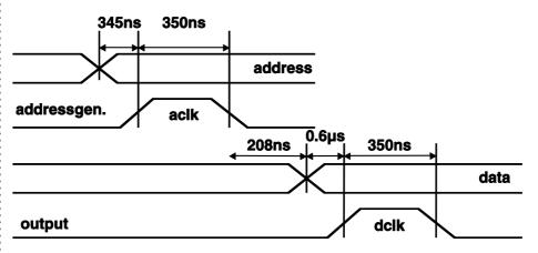
Input timing of extended I/O system (TINY-Tiger 2):
